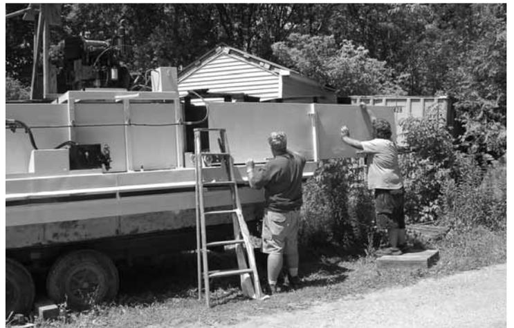
Workers sand and paint the Aquarius System EH-420 which, along with other needed repairs, will extend the functional life of the SAAWA harvester.
