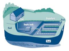
polyethylene. The tank holds the water long enough to allow all solids to settle out (forming sludge) and oil and grease to float to the surface (as scum). Compartments and a T-shaped outlet in the septic tank prevent sludge and scum from leaving the tank. Screens are also recommended to keep solids from entering the drainfield.
