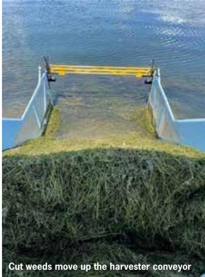
Cut weeds move up the harvester conveyor
